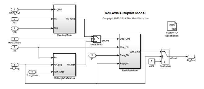
The rtwdemo\_roll model implements a basic roll axis autopilot algorithm, which controls the aileron position of an aircraft.
