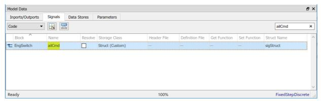
7 Use the **Filter Contents** box to search for the **phiCmd** signal. Configure the signal to use the same structure variable, **sigStruct**.
