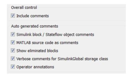
In the model roll, "Include comments" (Simulink Coder) is selected to include comments in the generated code and enable the other comment parameters. If you configured
